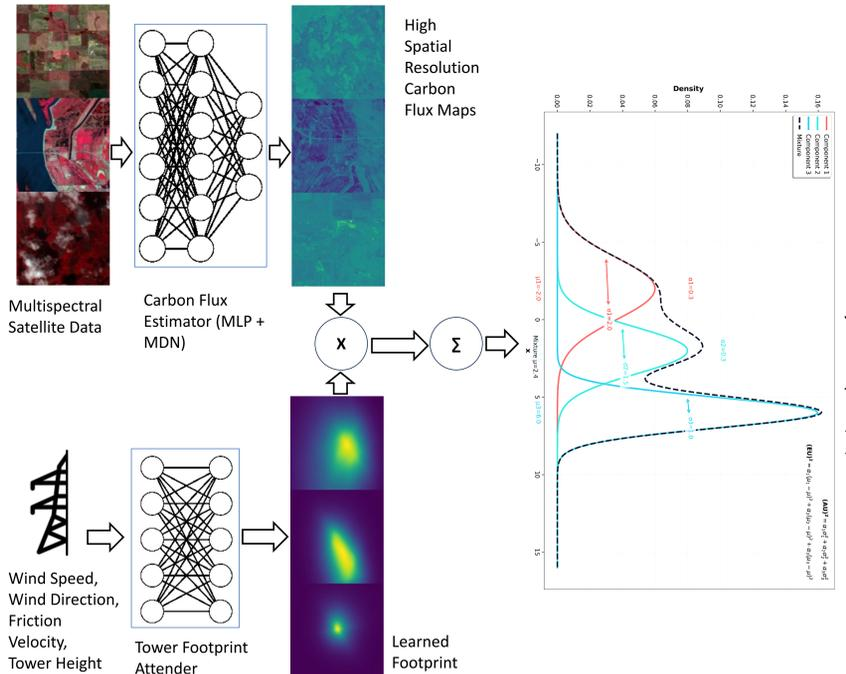
Figure: MDN-based architecture combining Landsat and meteorological inputs for carbon flux prediction and uncertainty estimation.
